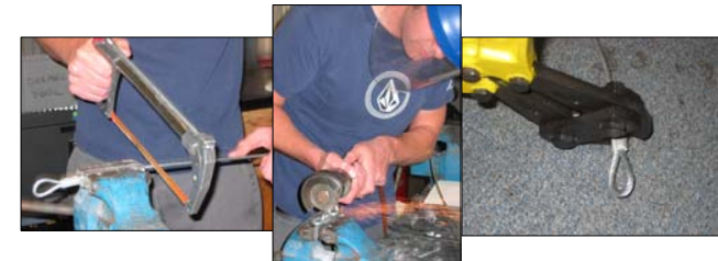
Figure 6. Testing the locking device of the improved design against the benchmark with (a) a hacksaw, (b) a pneumatic grinder, and (c) bolt cutters.
